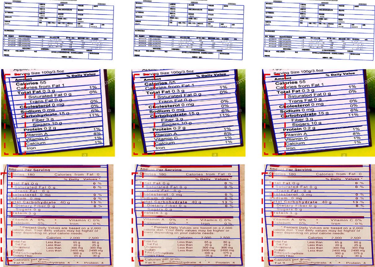
Fig. 16. Some table structure recognition results obtained by TSRFormer and SEMv2 on the WTW dataset. First Column the table structure predictions from the TSRFormer. Second Column the table structure predictions from the SEMv2. Third Column the ground truth table structure. The red dash boxes denote the different prediction regions between TSRFormer and SEMv2.
