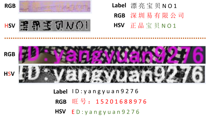
Fig. 5. Illustration of the benefits of HSV channels. Two text line images are difficult to recognize via RGB representations, but the representation can be improved by using HSV channels. The red "H" denotes that the image is the visualization of the H channel, while the red "S" denotes the S channel. The groundtruth, recognition results without HSV channels and recognition results with HSV channels are shown right behind "Label", "RGB" and "HSV".
